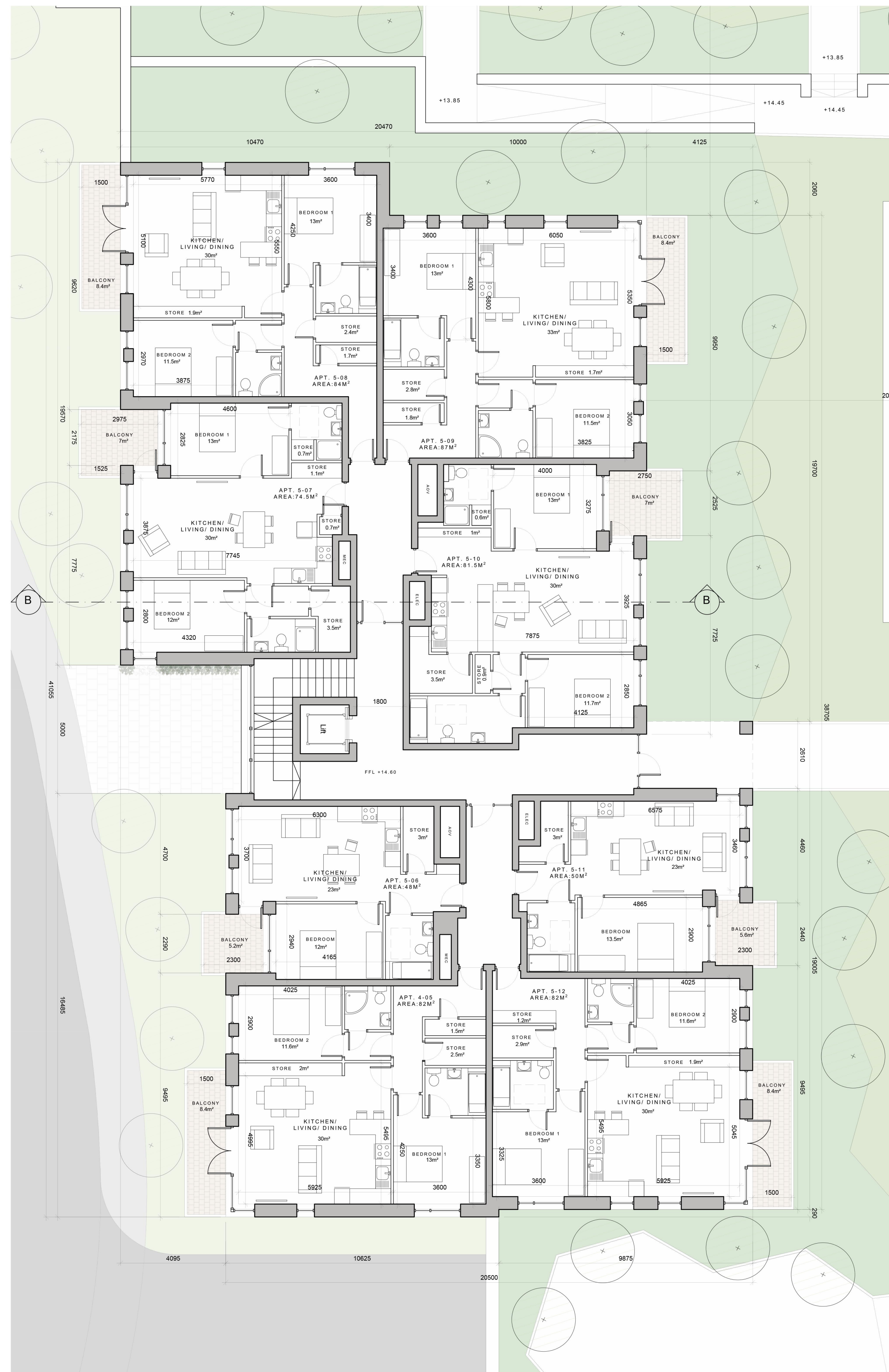
BLOCK 5 FIRST FLOOR PLAN SCALE: 1:100 SEE THE BIG SPACE LANDSCAPE ARCHITECTS DRAWINGS FOR DETAIL OF LANDSCAPE TREATMENT
