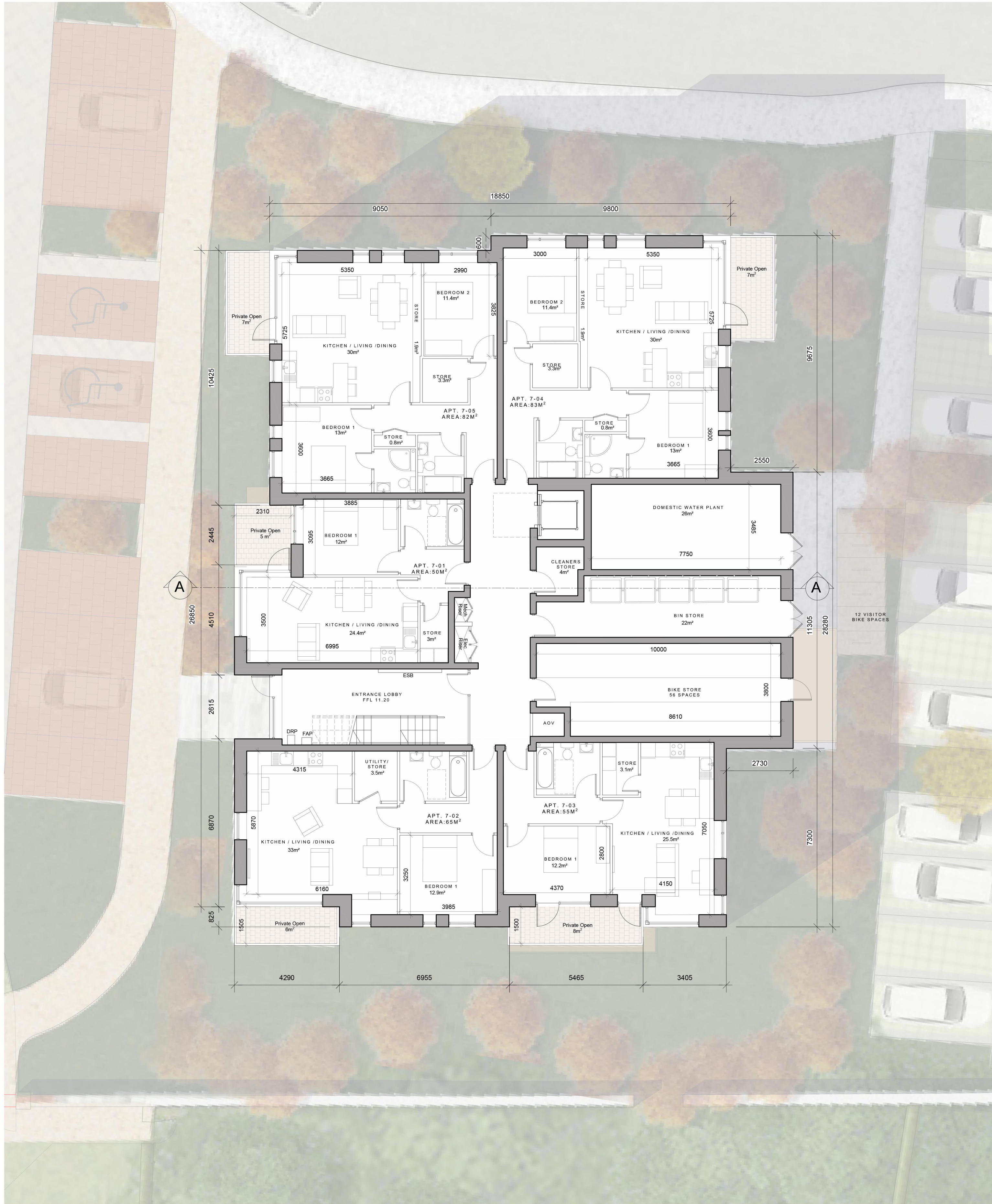
BLOCK 7 GROUND FLOOR PLAN SCALE: 1:100 SEE THE BIG SPACE LANDSCAPE ARCHITECTS DRAWINGS FOR DETAIL OF LANDSCAPE TREATMENT
