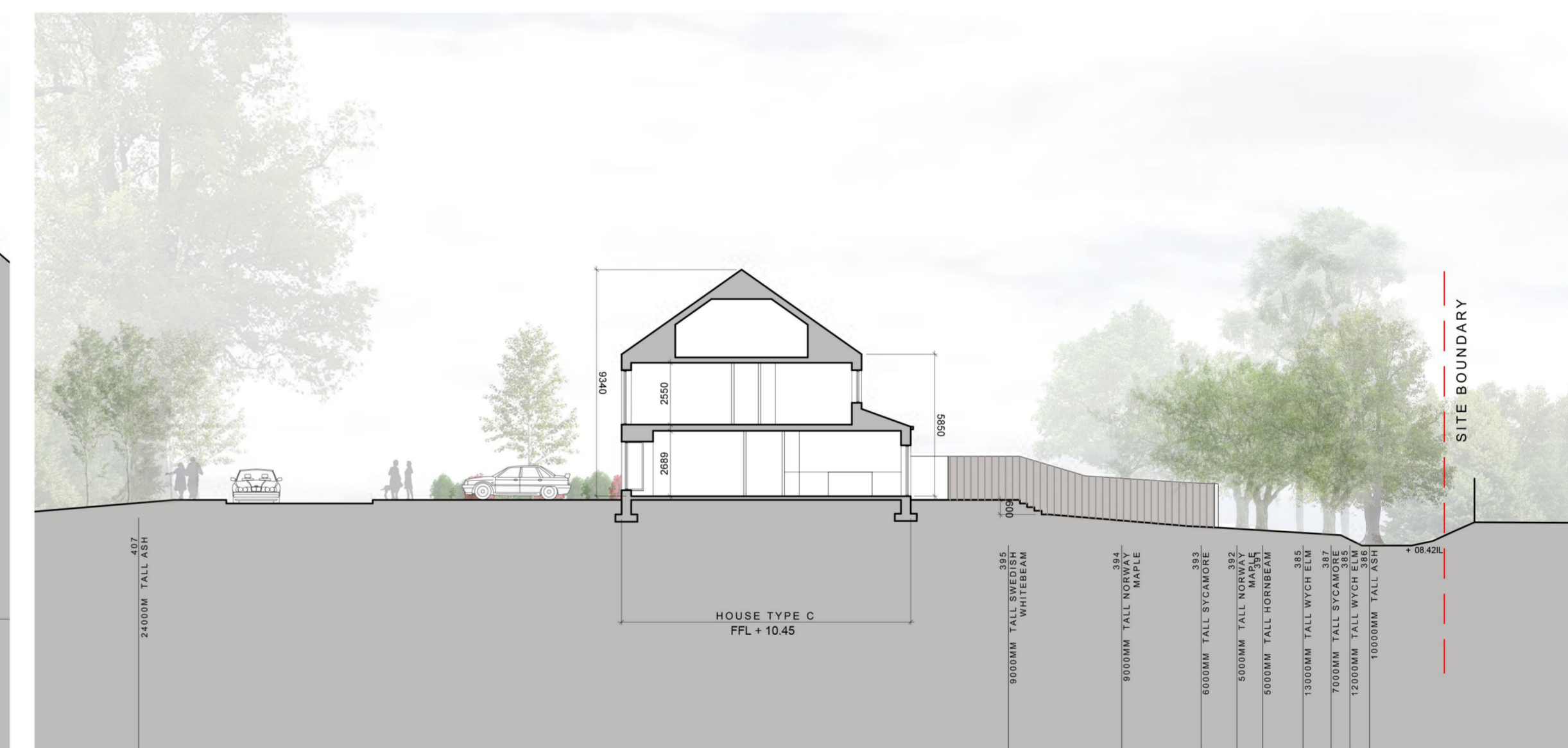
SITE SECTION 4 - 4 SCALE: 1:200 NOTE: SEE LANDSCAPE ARCHITECTS DRAWINGS FOR BOUNDARY TREATMENTS SEE ARBORISTS REPORT FOR DETAIL ON EXISTING TREES DOTTED RED LINE INDICATES SITE BOUNDARY
