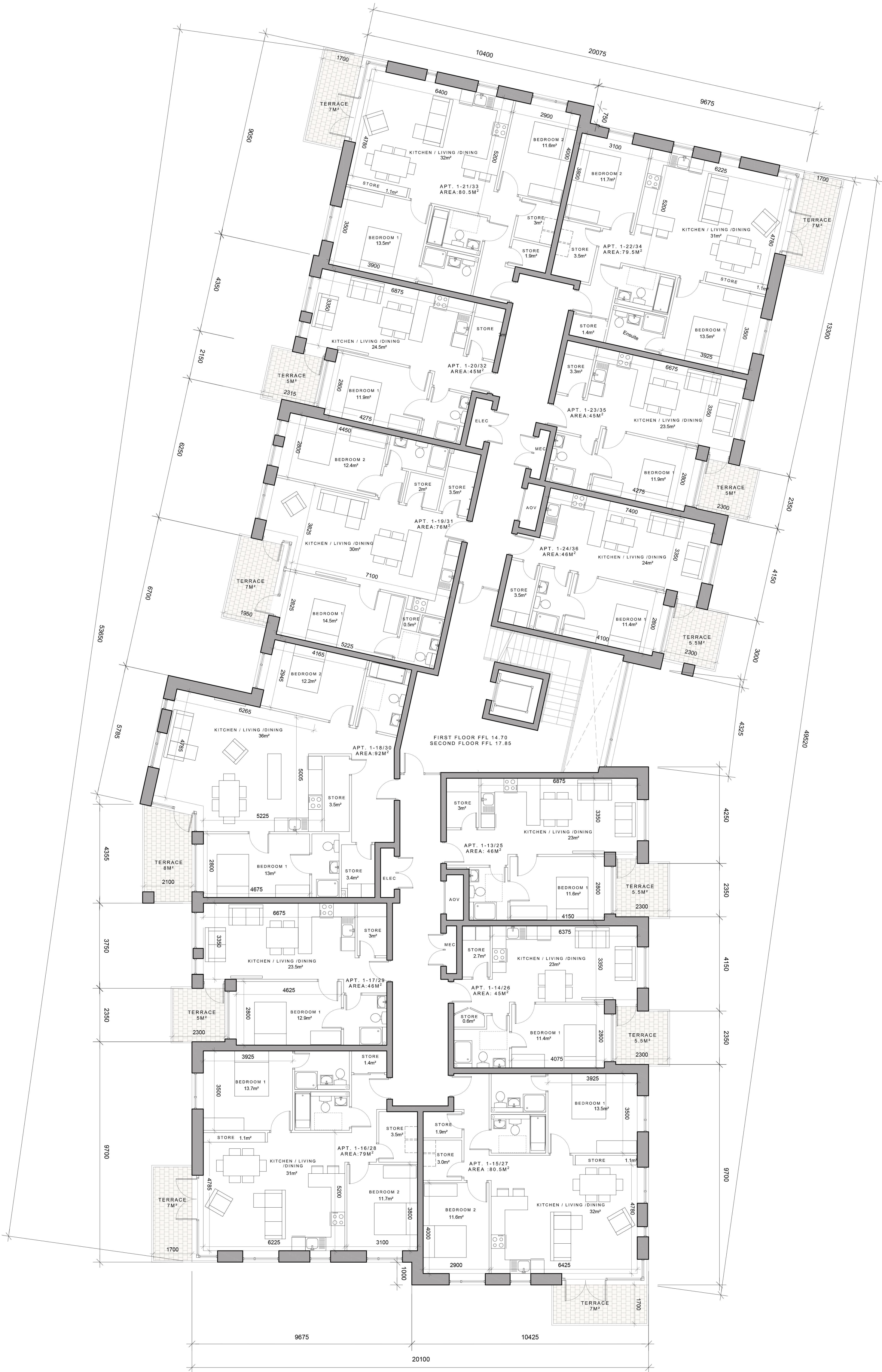
BLOCK 1 FIRST / SECOND FLOOR PLAN SCALE: 1:100
